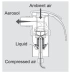
The size of the aerosol droplets is determined by the nozzle inserts. The smaller the droplets are, the farther they can penetrate into the deeper and smaller regions of the lung:
